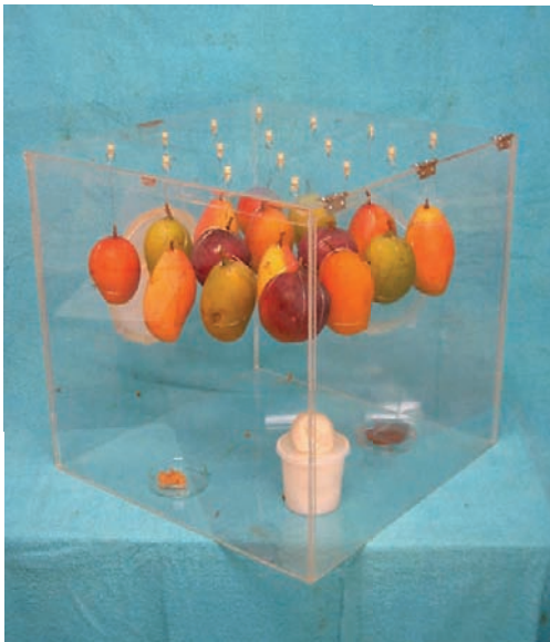
Figure 1. Acrylic cage with mango fruits hung from the top, used to test varieties under artificial infestation of A. obliqua .
